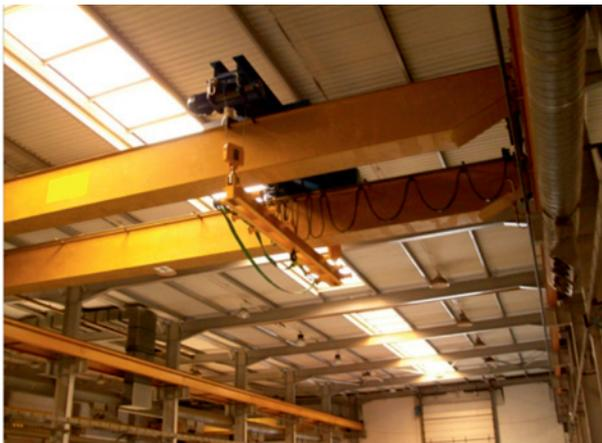
The system worked exceptionally well due to the stability of the lifting beam and the ease of slinging to the designated points along the beam, loads can be slung and transported by a single operator in a controlled and safe manner.
