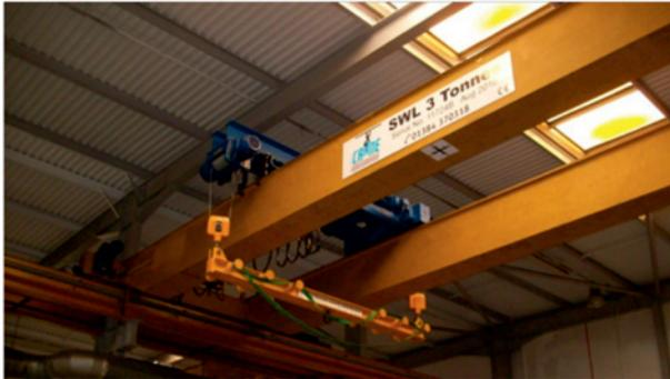
Both cranes were fitted with Flex radio control to allow either "Hoist A", "Hoist B" or "Hoists A and B" to be operated, allowing the operator to adjust an uneven load if required.
